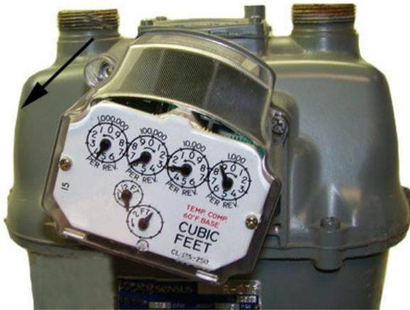
2. Install and tighten endpoint-to-meter mounting screws in an alternating fashion.
