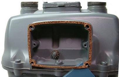
**To assemble the 100G Datalogging gas endpoint and index**
